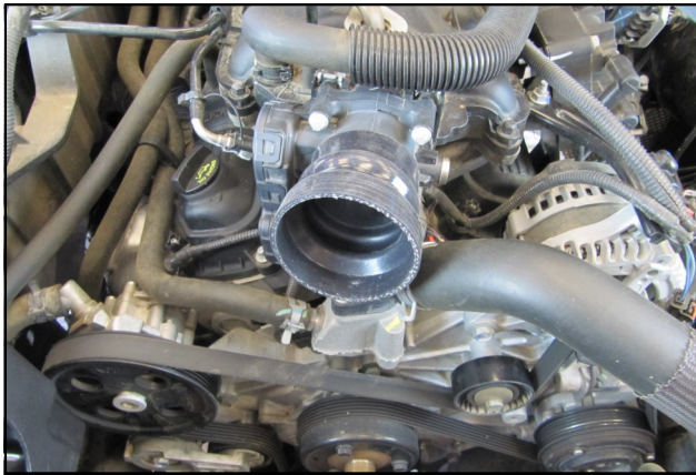
10. Slip the Hump Hose Coupler (#5) onto throttle body WITH OUT the clamps at this time.
